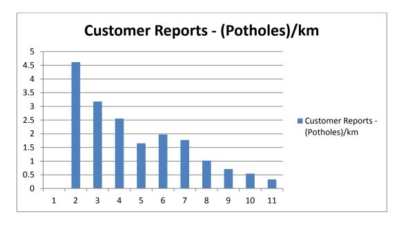
47. The customer reports information indicates that there are more pothole defect reports per kilometre for the higher type roads, with the highest rate being on the Type 2 roads.
