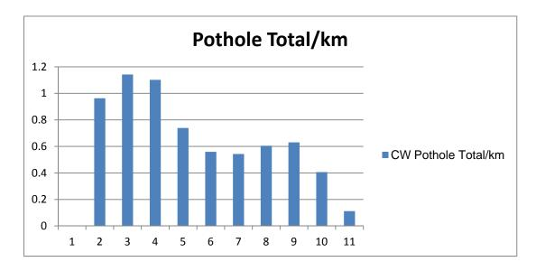
43. The Type 2, 3 and 4 roads have higher rates of potholes per kilometre compared to the other road categories. However, it is noticeable that the number of potholes per kilometre for the more serious safety defects (P1 potholes) is significantly higher on the Type 2, 3 and 4 roads than on the other road categories.
